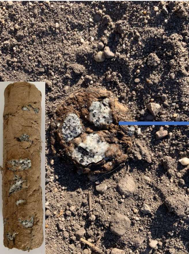
50 mm diameter granite SVD in industrial soil
