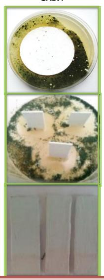
A simple comparative experiment shows that in terms of pathogenic fungi GALVI paint containing microcells of zinc and copper is much more effective than paints containing hazardous biocides (eg. Triclosan) as a fungicide.
